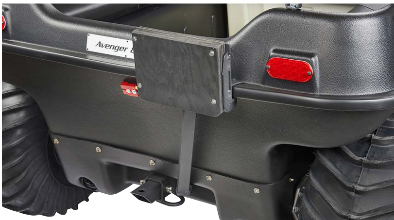
OUTBOARD MOTOR BRACKET RIGHT SIDE MOUNT 617-09
